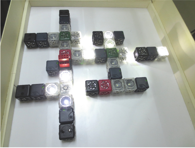
Fig. 5. Robotic binary adder with optical computation, inspired in competing patterns.
