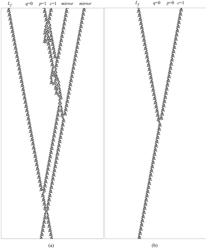
FIGURE 13 Fredkin gate in ECAM rule \phi_{R22maj:4} . (a) INPUT c = 1, p = 1, q = 0 , OUTPUT x = 1, y = 1, z = 0 , (b) INPUT c = 1, p = 0, q = 0 , OUTPUT x = 1, y = 0, z = 0 .
